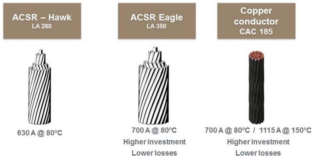
Figure 2 – Comparing three different types of overhead line conductors
