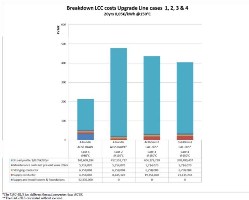
Figure 4 – Comparing the life cycle cost of a line refurbishment with a copper conductor and the same line refurbishment with an ACSR conductor
