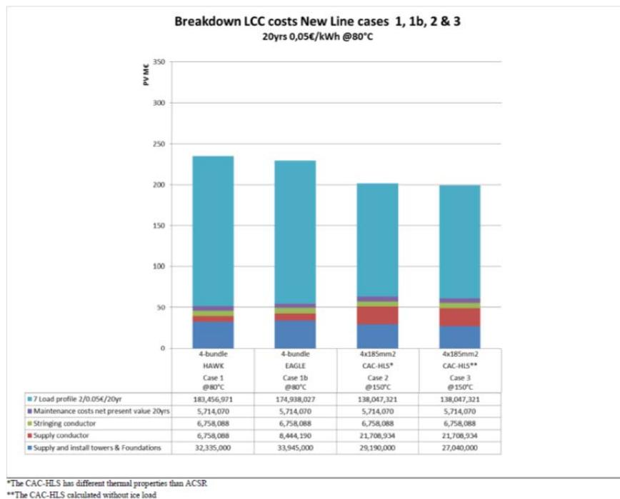
Figure 3 – Comparing the life cycle cost of a new line with a copper conductor and the same line with an ACSR conductor.
