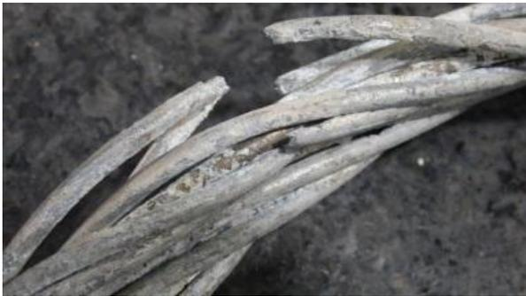
The characterization of the ACSR LA-56 conductor has been done by taking measurements of breaking strength and electrical resistance on the aluminum wires and the steel core. In addition, an estimation of the loss of mechanical and electrical features has been analyzed considering also the breakage of 4 from the 6 aluminum wires that constituted the ACSR LA-56 conductor. The obtained results have been compared with the reference values specified in the norm UNE-EN 50182:
