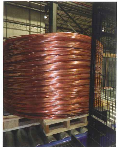
Typical copper coil weighing 5 tonnes
