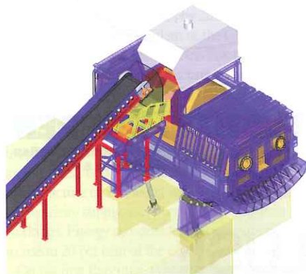
The design concept of the Refining Furnace type FR 250 with loading from the top
