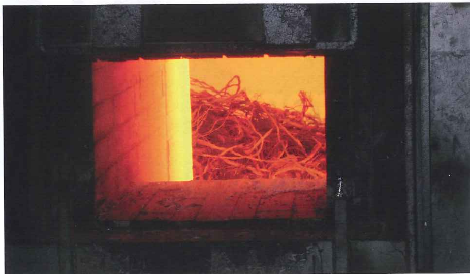
View of the scrap inside the Refining Furnace type FR 250
